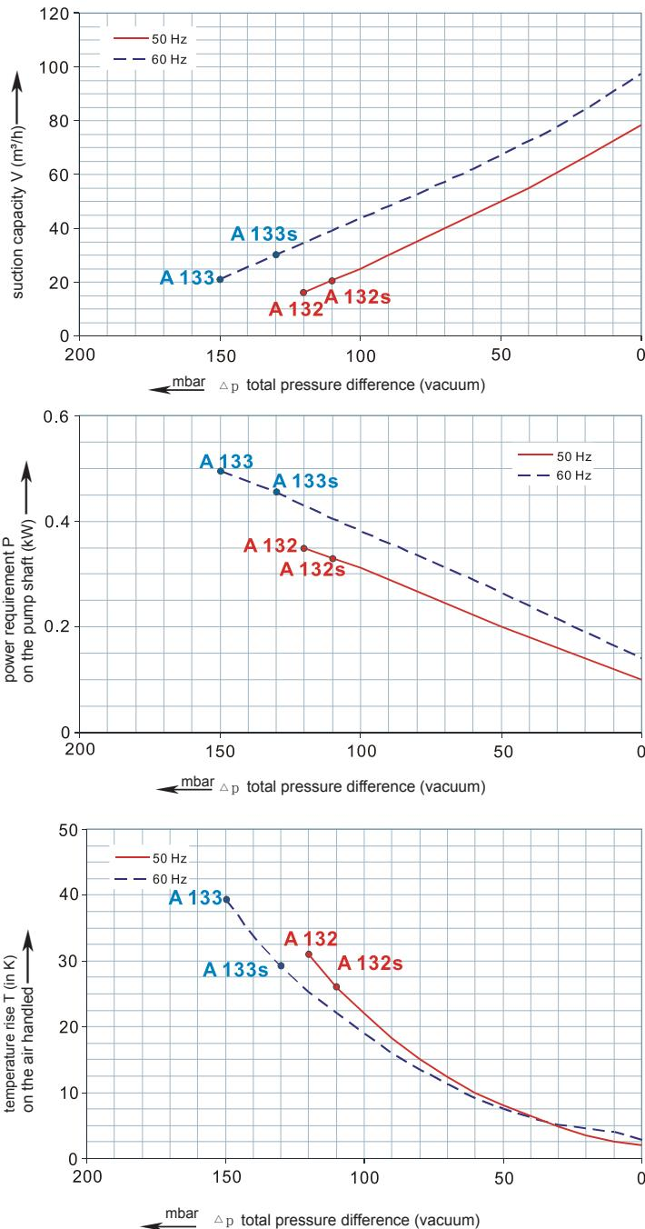
The performance curves are based on air at a temperature of 15 °C and an atmospheric pressure of 1013 mbar with a tolerance of +/- 10 %.
